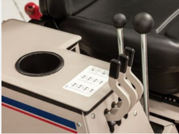
Control Levers for the 3-Point Hitch
